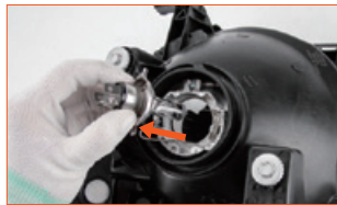
Fig. 1: Remove the dust cover and the OE Halogen bulb. Hold the base of the lamps and turn counter-clockwise until it is unlocked, and then remove the OE Halogen bulb;
