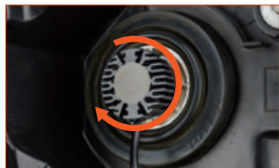
Fig. 3: Insert the lamps , turn them clockwise, then clamp tightly.
