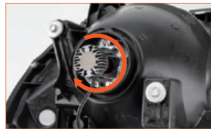
Fig. 4: Rotate the base of the lamps clockwise until it is in the correct position;
