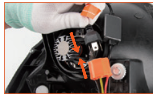
Fig. 5: Please double check the “+/-” polarity before connecting the plug. (Only apply for a few models).
