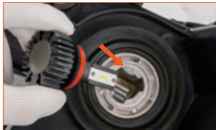
Fig. 2: Line-up the retainer holder with the slot of the assembly.
