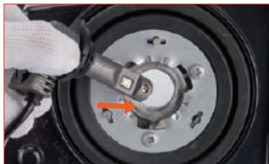
Step 2: Line-up the retainer holder with the slot of the assembly.
