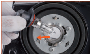
Step 1: Remove the dust cover and the OE halogen bulb.
