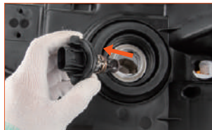
Step 1: Remove the OE halogen bulb
