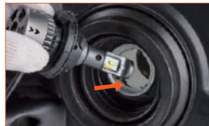
Step 2: Insert 9008/H13 into the assembly and rotate it clockwise, then lock it.
