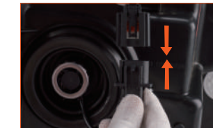
Fig. 3: Connect the power line.
