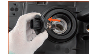
Fig. 1: Remove the OE halogen bulb
