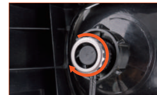
Fig. 5: Rotate the heat sink to make it tight (If the high beam and the low beam reverse, take the bulb out and rotate it 180 degree,and then install it again.)
