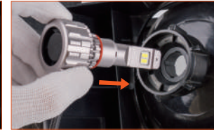
Fig. 4: Insert the lamps into the retainer holder with correct position.
