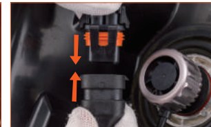
Fig. 4: Connect the power line.
