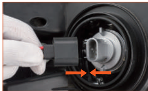
Fig. 3: Connect the power line.
