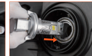
Fig. 2: Insert 9008/H13 into the assembly and rotate it clockwise, then lock it.
