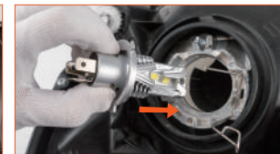
Fig. 2: Insert the LED lamps into the assembly slot, match the tabs with slot, and lock the LED lamps with the buckle.
