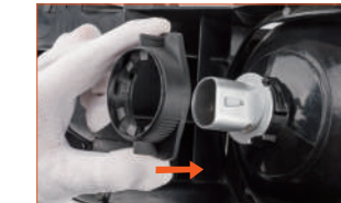
Fig. 3: Then insert them into the assembly.
