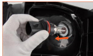
Fig. 1: Remove the bulb retainer and OE halogen bulb from the vehicle.
