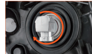
Fig. 3: Insert the lamps , turn them clockwise, then clamp tightly.
