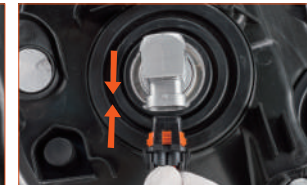
Fig. 4: Connect the power line.
