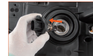
Fig. 1: Remove the OE halogen bulb
