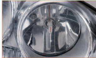
Step 4: When the LED bulb is fixed, the two sides equipped with LED lamp beads should face the direction of 3-9 o'clock
