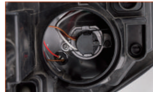
Step 4: Connect the LED bulb plug to the original vehicle socket
