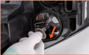
Step 1: Remove the original car plug, open the spring clip, take out the original light bulb
