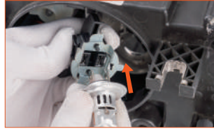
Step 2: Insert the led bulb into the original adapter
