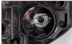
Step 3: Fix it in place with a spring clip
