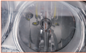
Step 5: When the LED bulb is fixed, the two sides equipped with LED lamp beads should face the direction of 3-9 o'clock respectively
