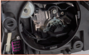
Step 3: Insert the LED bulb into the assembly, put the tabs of the locking ring opposite to the slot of the assembly, and tighten it in the assembly
