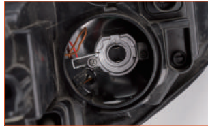
Step 2: Insert the LED bulb into the assembly and align the tabs of the ring with the slot of the assembly
