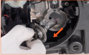
Step 1: Remove the original car plug and take out the original light bulb
