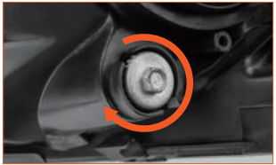
If the beam pattern is too high, adjust the buckle of the assembly to adjust the beam pattern. (As the picture shows above.)
