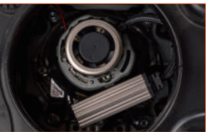
Fig. 4: Sort and fix the wiring harness with Zip Ties or Double-side Tape. You can also insert the drive into assembly.
