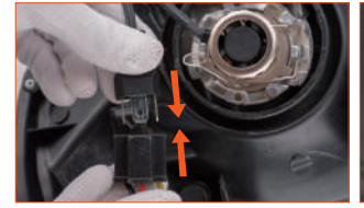
Fig. 5: Please double check the "+/-" polarity before connecting the plug. (only for H7).
