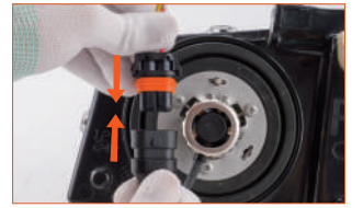
Fig. 4: Connect the power line.
