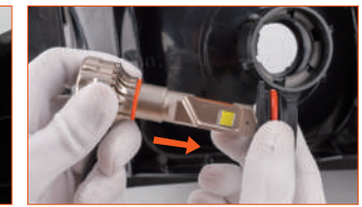
Fig. 2: Take apart the retainer holder from LED lamps.
