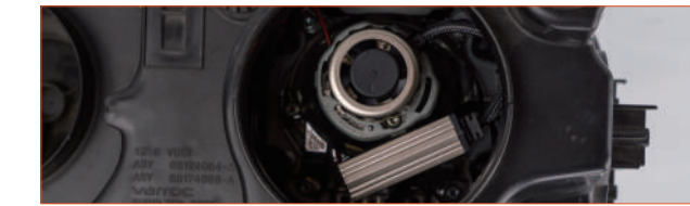
Fig. 5: Sort and fix the wiring harness with Zip Ties or Double-side Tape.You can also insert the drive into assembly.
