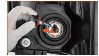
Fig. 1: Remove the dust cover and the OE halogen bulb.
