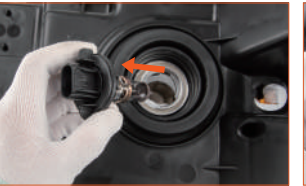
Fig. 1: Remove the OE halogen bulb
