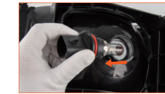
Fig. 1: Remove the bulb retainer and OE halogen bulb from the vehicle.
