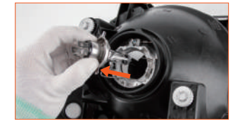
Fig. 1: Remove the dust cover and the OE Halogen bulb. Hold the base of the lamps and turn counter-clockwise until it is unlocked, and then remove the OE Halogen bulb;
