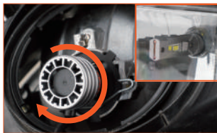
Fig. 4: Rotate the heat sink to get a better beam pattern (It will get a best beam pattern if the LED chips face 3-9 o'clock.)
