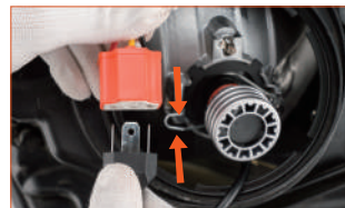
Fig. 5: Please double check the "+/-" polarity before connecting the plug. (only for H7).
