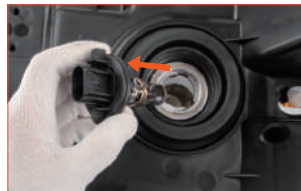
Fig. 1: Remove the OE halogen bulb.
