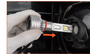
Fig.3: Insert the lamps into the retainer holder with correct position.
