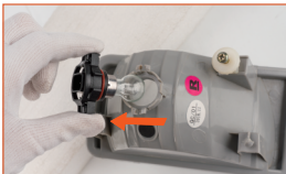
Fig.2: Press the tabs on both sides of the halogen bulb and remove the original bulb.
