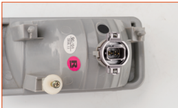
Fig.4: Push the snap ring without rotating, ensuring that the assembly is fully aligned in the correct position without any looseness.
