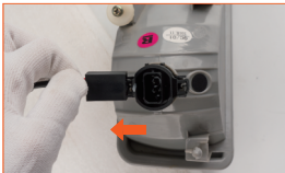
Fig.1: Remove the bulb compartment rubber cover and disconnect the original vehicle connector.
