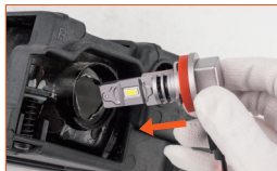
Fig.3: Line-up the tabs with the slots of the assembly (Warn: the tabs are asymmetrical)
