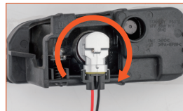
Fig.4: Insert the lamps, turn them clockwise and clamp tightly
